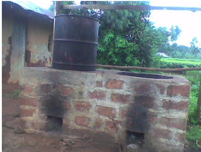
The stalked substrate bags are placed in the drum which is heated for a period of 45 minutes.
